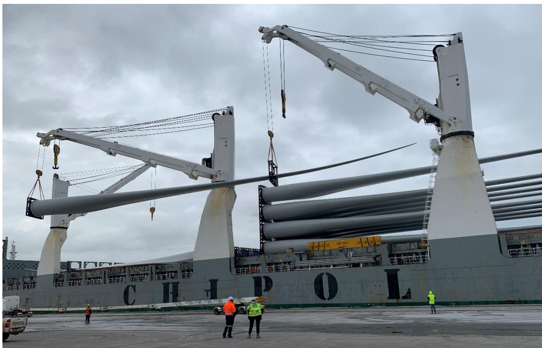
Figure 1: Stevedoring workers in Geelong perform a dual lift of a 100 tonne wind turbine blade using two ship's cranes. The blades were transported to onshore wind projects in western Victoria.
